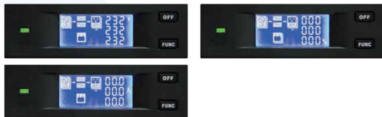
DC bus and battery voltages (positive and negative) & current
